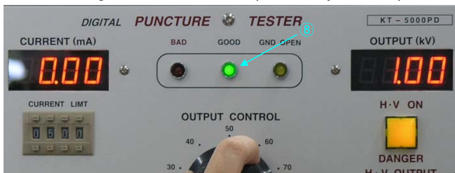
Fig 2) Green Lamp showing good test result
