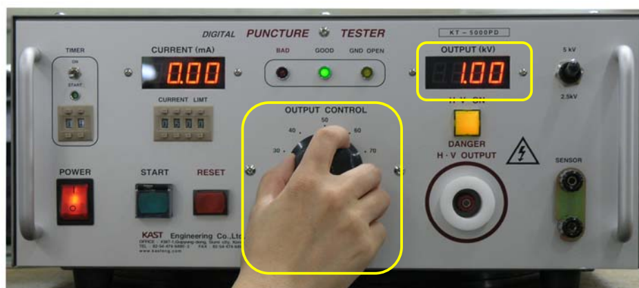
Fig 3) Adjusting of test voltage
