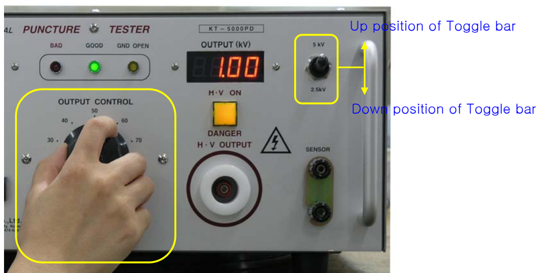
Fig 4) Adjusting of OUTPUT VOLTAGE KNOB
